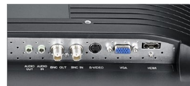
Video versatility, including VGA, HDMI, S-Video and BNC In/Out
