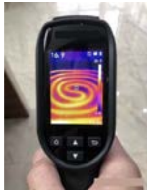
Check Floor Heating
